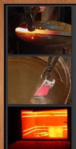
The hot steel is beaten into shape with a hammer and anvil.
